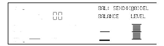
There are only two parameters: Balance and Input Level. This is because in Configuration #1, effect send 4 only has a Delay effect, and not a Pitch effect like the other effect sends do. Quad Knob [1] controls the Balance between the Delay output and the dry effect send signal, while Quad Knob [3] controls the overall input level to the Reverb.
