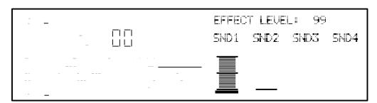
Note: If a Sound is not enabled in a Program, its title will be shown in lowercase ("snd4"), and adjust its controls will have no effect on the Sound until the Sound is enabled. To enable a Sound, hold down its respective Quad Button (i.e., [3] for Sound #3) and press VALUE [ ].
