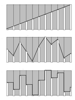
*Tip:* The Tracking Generator can be used to turn a variable control, such as the Mod Wheel or velocity, into a switch by setting all of the points to 0 except for point 10. Only near the maximum input will anything other than 0 come out of the Tracking generator. You can patch the Mod Wheel somewhere else in addition to the Tracking Generator, giving you gradual control of one function with the full range of the Mod Wheel, while switching on a second function only at the top of the wheel.
