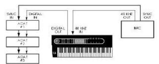
$\it Tip:$  With this type of connection, the ADAT tracks will remain in tune with the QuadraSynth Plus even when the BRC's pitch value is adjusted.
