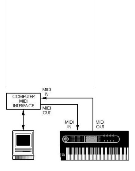
If you are driving other MIDI gear (such as an expander module or MIDI-responsive signal processor), you'll usually drive these from the sequencer if it has additional MIDI outputs. However, you can also use the QuadraSynth Plus's MIDI THRU connector to drive other modules since the Thru carries a replica of what appears at the QuadraSynth Plus's MIDI IN, which is the same as the sequencer's MIDI OUT.
