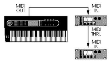
To drive MIDI controlled devices from the QuadraSynth Plus, patch the QuadraSynth Plus's MIDI OUT to the MIDI device's MIDI IN. If there is more than one MIDI device, patch the first device's MIDI THRU to the second device's MIDI IN, the second device's MIDI THRU to the third device's MIDI IN, etc.
