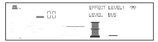
Turn Quad Knob [1] to adjust the effect send level of the selected Sound (1—4).
