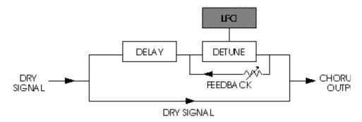
**Stereo Chorus.** In the case of a Stereo Chorus, the signal is split into three parts with a dry signal and a separate Detuning section for both left and right channels. When the left channel is detuned sharp, the right is detuned flat, and vice versa. Once again, this causes the effect to become more pronounced and dramatic.
