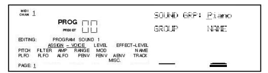
The Assign Voice function is the most fundamental part of Program editing. It is where you choose the particular sample that forms the basis of a sound. To avoid scrolling through long lists of samples (remember, there are 24 megabytes of sounds in here!), sounds are divided into groups. After selecting the group, you then select the sample within the group.
