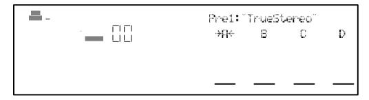
The current PROGram number is displayed, and the Program's name appears in the top-right. The current Bank is shown to the left of the Program name. The current MIDI channel is shown in the top left corner left.
