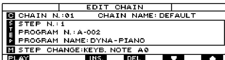
The display shows the number and name of the current chain, while the central window contains the number of the step and the corresponding program or patch with the relative number. The lower part of the display indicates the way in which the system moves forward through the steps, while the bottom line contains the usual icon rectangles corresponding to the function keys.
