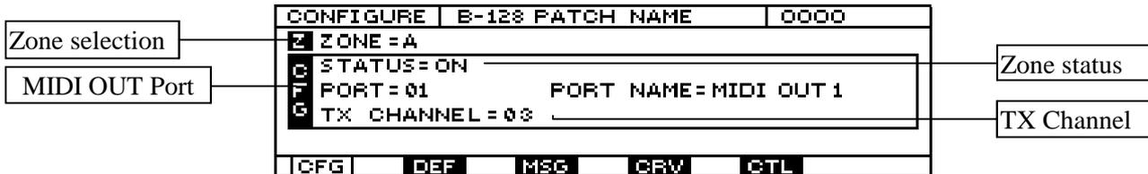
The name CONFIGURE, representing the second section name, the name of the current patch and the lights indicating the activation status of its zones all appear at the top of the display. Immediately below is a field where the user can select the individual zone of the patch to be set up. To do this, the user uses the cursor keys to locate on the ZONE= field and then selects the zone desired using the INC and DEC keys or the encoder.
