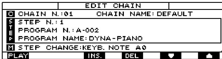
3. Press function key F6 to actually assign the selected patch to the current step. At this point, the step will automatically set on step n. 2.
