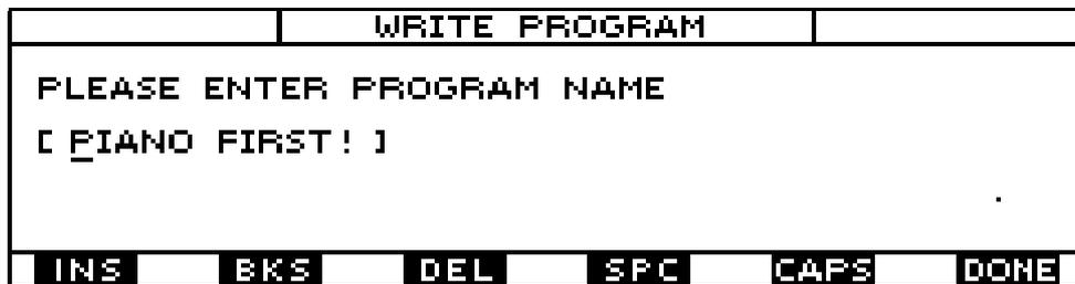
A dash blinking under the first character of the name indicates that this character is selected and can be modified using the data input devices (including the number keypad). The cursor keys can be used to locate on other characters and modify them with the same procedure, thus making up the new patch name. The function keys enable the following functions:
