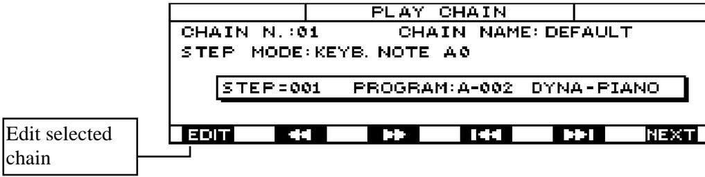
1. Press function key F1 (EDIT) to obtain the EDIT CHAIN page on the display; the PROGRAM N.: field is automatically selected, indicating the patch which corresponds to step 1 of the selected chain.
