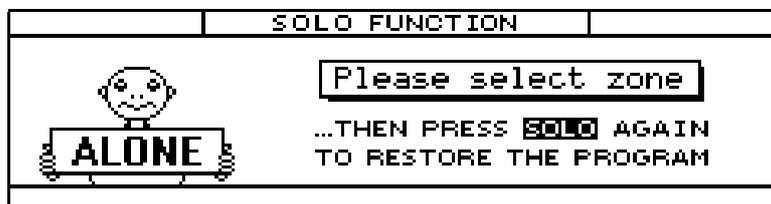
All the LEDs relating to the active zones will start to flash awaiting the selection. Press the key for the zone to be left active and the MC-3000 will return to the Top Page, switching all the other zones to Stand-by mode; when function key F6 (SOLO) is pressed again, the patch will be restored to the basic conditions.
