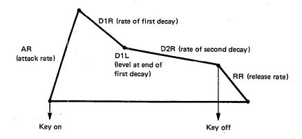
The following EG curves show the parameters for some common instruments. When creating voices on the DX21 you should apply these EG curves to the carrier operator.
