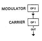
The bottom operator of a stack is called a CARRIER. Any operators which are connected to the carrier's inputs are called MODULATORS. YOU CAN'T HEAR A MODULATOR DIRECTLY, but you hear its effect by listening to the carrier's altered (modulated) output. A given operator can be either a carrier or a modulator: the only difference is how it is "connected" in a given algorithm.
