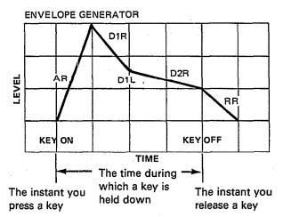
This envelope diagram can be used as a guide in visualizing DX21 envelope settings while you program or edit a voice.
