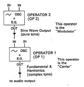
Operators do not have to be connected "vertically" in a modulator-carrier relationship, as shown above. The outputs of two operators can also be mixed—just as the stops in an organ are mixed. In this case the sounds are simply added together with no modulation effect.
