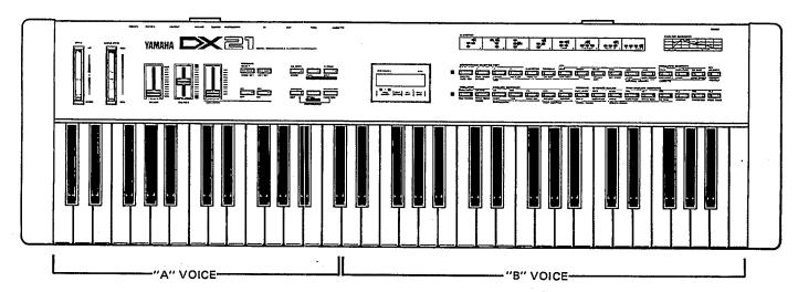
The split point number on the LCD will change to the number of the pressed key, the "A" voice will be playable on all keys to its left (Including the split key), and the "B" voice will be playable on all keys to the right of the split key. This process can be repeated as many times as necessary, but you must press and hold the S POINT key again every time you re-program the split point.
