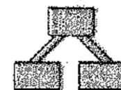
Next, we will consider the form where there are, again, multiple carriers, but now each is modulated by the same modulator, as is the case in algorithm No. 22 of the synthesizer, where operators 3, 4, and 5 are carriers modulated by operator 6 (Fig. 6.2). In this case we consider each carrier separately and compute the spectrum as we did above. With this algorithm we can exactly duplicate the spectrum of Fig. 6.1 and have two operators left over.
